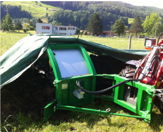
TG 201 during work with fleece underpassing.
