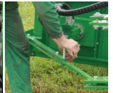
Locking after swiveling the tunnel
